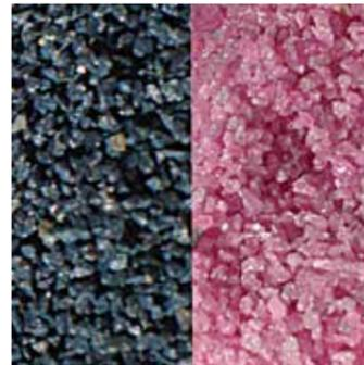
Coarse grit is intended for coarse grinding, in which large material removal rates are required, while finer grit is intended for achieving smooth surfaces and for small material removal rates.
